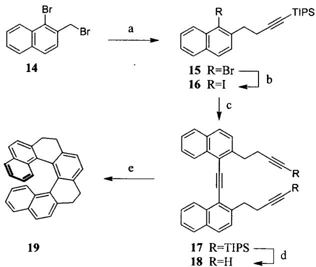
**Scheme 3.** (a) LiCH<sub>2</sub>C≡CTIPS (1.2 equiv), THF, -78 °C, 3 h, 71 %; (b) n-BuLi (1.1 equiv), THF, -78 °C, 0.5 h, then I<sub>2</sub> (1.1 equiv) in THF, -78 °C to rt, 0.5 h, 92 %; (c) gaseous HC≡CH, Pd(PPh<sub>3</sub>)<sub>4</sub> (5 mol %), CuI (10 mol %), piperidine, 80 °C, 2 h, 77 %; (d) n-Bu<sub>4</sub>NF (4 equiv), THF, rt, 1 h, 70 %; (e) CpCo(CO)<sub>2</sub> (20 mol %), PPh<sub>3</sub> (40 mol %), decane, irrad., 140 °C, 2 h, 64 %.
